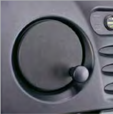
Steer tiller handle position and steer effort are adjustable to help reduce operator fatigue.
