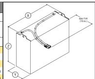
Battery Compartment is designed to accommodate standard wet cell batteries with fixed lifting eyes and no cover.
