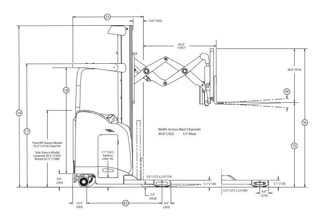
Circled dimensions correspond to the line numbers on the tabulated chart inside the Technical Guide. Dimensions are in inches (millimeters).
