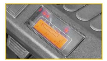
A newly developed LC instrument panel displays the full truck status, relevant fault codes and other important information, providing owners and operators with a clear and convenient understanding of the trucks health ensuring easy maintenance can be carried out when necessary.
