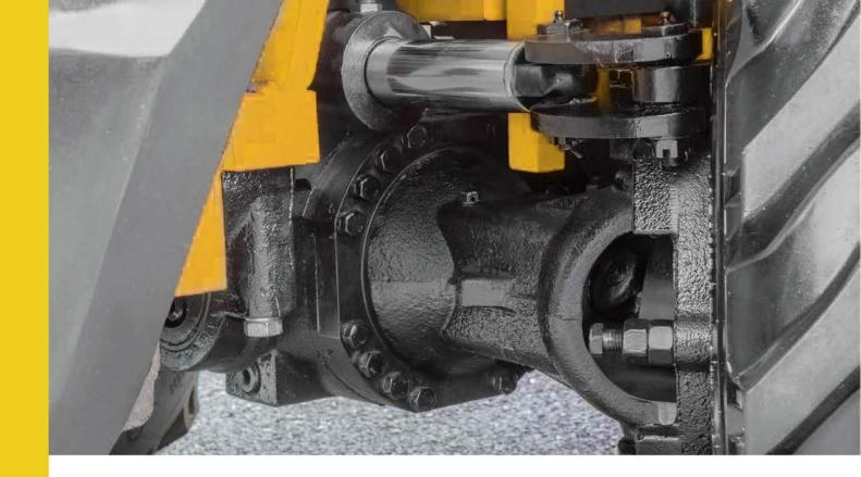
Individual oscillating steer axles allow each wheel to drive over obstacles, whilst keeping the truck and load level.
