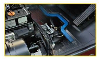
In addition to rubber dampening between the forklift frames and steering axles, compound engine dampening and a full floating power train provide a flexible connection, significantly reducing vibrations from the driving system.
