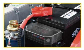
Adoption of a new generation integrated electric box allows for easy maintenance and repairs. The unit also provided improved water-proof protection.
