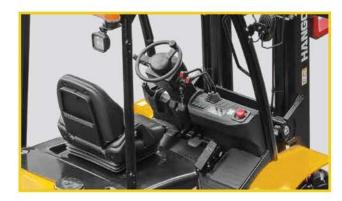
Extra space in the foot well significantly reduces operator fatigue, non-slip floor covering allows for easy and safe entry and exit from the cabin. The newly designed steering wheel, brake system and easy to operate levers provide improved handling.
