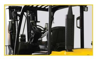
Increased forward visibility results from the broader mast design with a larger gap between the inside mast.
