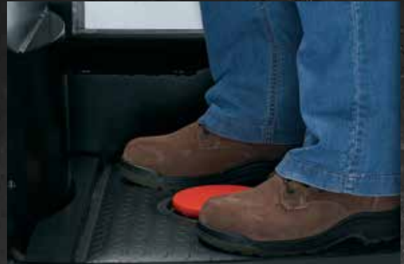
Multi-zoned operator presence floor system
