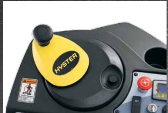
Adjustable steering tiller
