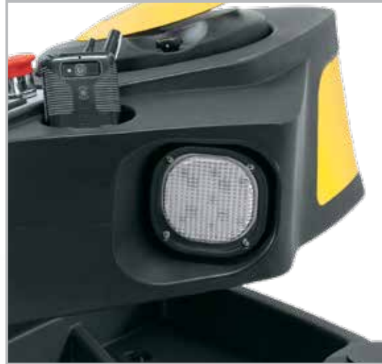
Optional LED work light with ultrasonic sensor
